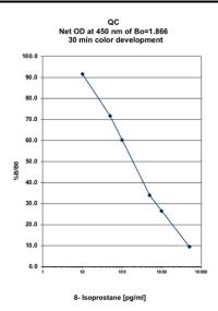
The data shown here is an example of typical results obtained using the Detroit R & D 8-isoprostane ELISA kit. These results are only a guideline, and should not be used to determine values from your samples. The user must run their own standard curve every time.
